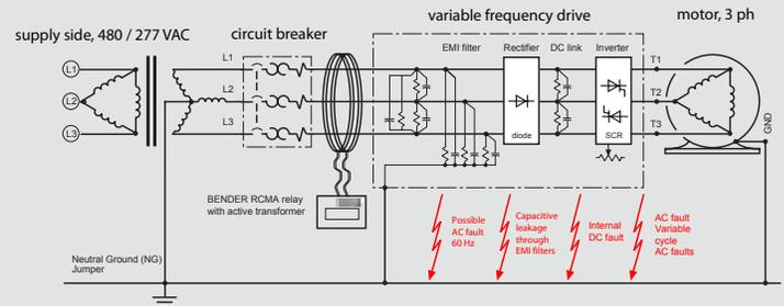
Figure 7: Grounded system with variable frequency drive
