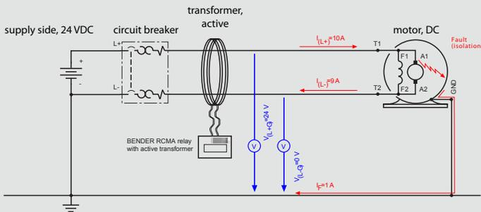
Figure 6: Grounded DC power system
