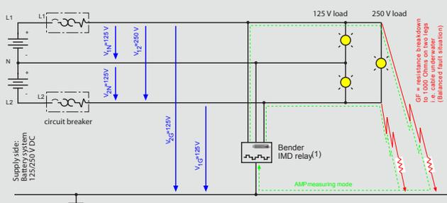
Figure 3: 125/250 VDC ungrounded system with IMD
