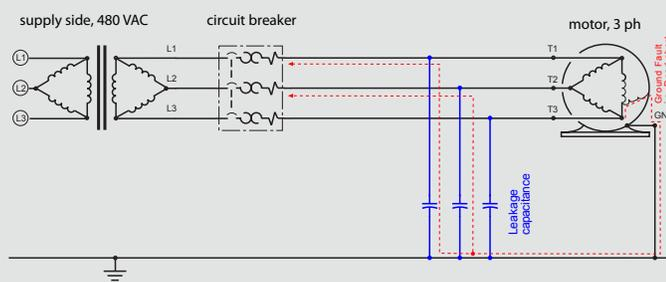
Figure 1: Ungrounded system in single-fault condition
