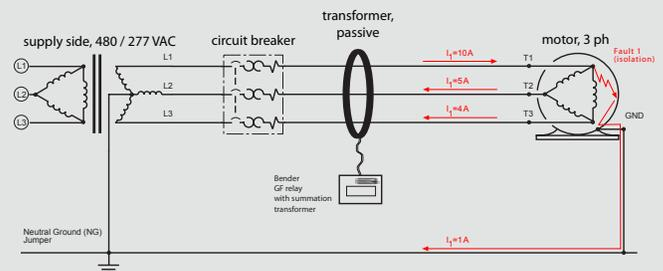
Figure 5: Faulted three-phase grounded system with zero-sequence relay
