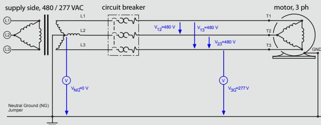
Figure 4: Simplified wye-configured, 480/277 V three-phase system
