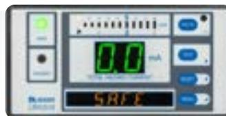
Bender's LIM2010 is ideal for retrofitting applications regardless of the current LIM's make and model. For the majority of applications, no metal cutting is needed and simple instructions facilitate a fast changeover. Its automatic self-calibration, self-check and digital display allow for yearly performance testing as opposed to bi-annual testing for analog LIMs (per NFPA 99).
