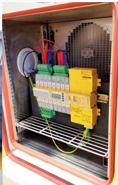
ATICS® during testing temperature test -25°C
