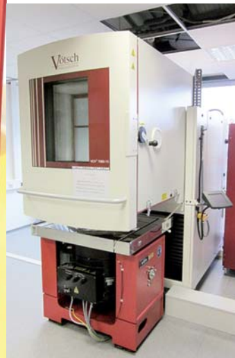
EMC test chamber in combination with vibration
