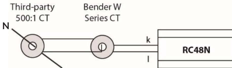
Fig 3: Cascaded CT connection example
