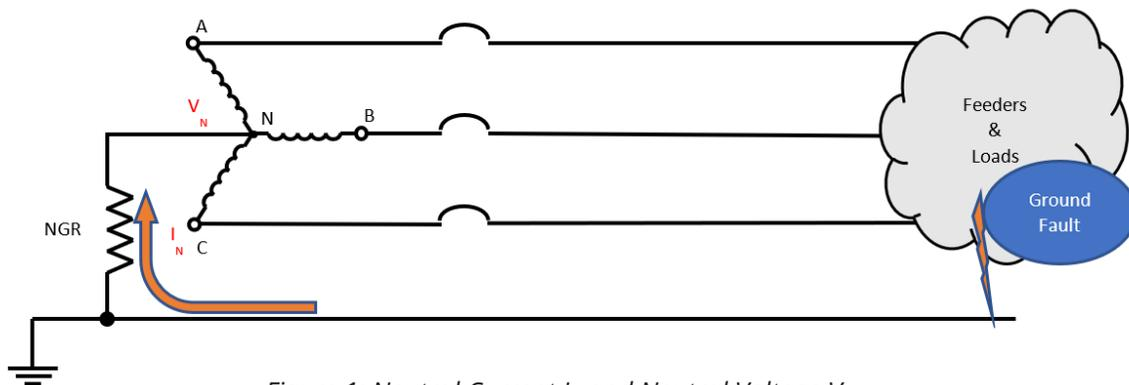
Figure 1: Neutral Current  $I_N$  and Neutral Voltage  $V_N$
