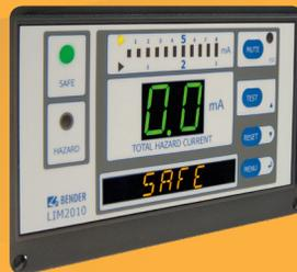
BENDER's LIM2010 is ideal for retrofitting applications regardless of the current LIM's make and model. For the majority of applications, no metal cutting is needed and simple instructions facilitate a fast changeover. Its automatic self-calibration, self-check and digital display allow for yearly performance testing as opposed to bi-annual testing for analog LIMs (per NFPA 99).
