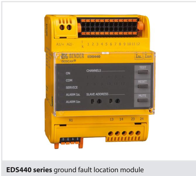
The EDS440 uses the latest in monitoring technology to locate ground faults in ungrounded AC and DC systems. Fault location takes place automatically while the system remains online, without the need to open branch breakers or disconnect equipment. Up to twelve branches can be continuously monitored from a single device.
